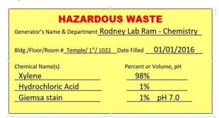
Make Sure the label is filled out with the Name of the Generator
